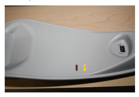
2. Read the link label on the bottom of the cradle with the scanner. The scanner will sound a good read beep and the LED will flash amber.
